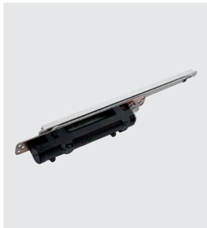
Completely invisible from the outside, it is installed into the door panel while the opening arm is fixed to the frame. It requires a milling to be machined on the header of the frame and on the upper edge of the door panel.
