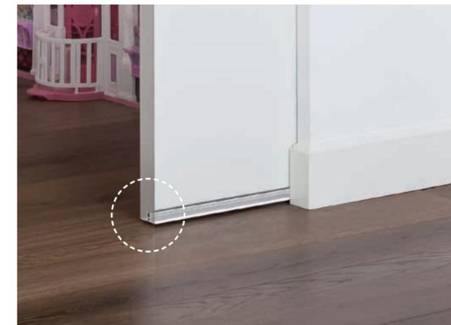
ECLISSE offers an extruded aluminium guide section, specifically designed and developed to be fitted into the bottom of sliding pocket doors. This profile is easy to fit even on an already installed pocket door, requiring no special processing apart from a milled recess along the lower edge of the door panel. The technical performances offered by the anti-warp profile are an improved sliding action, an increased wear resistance and protection against deformation due to humidity.
