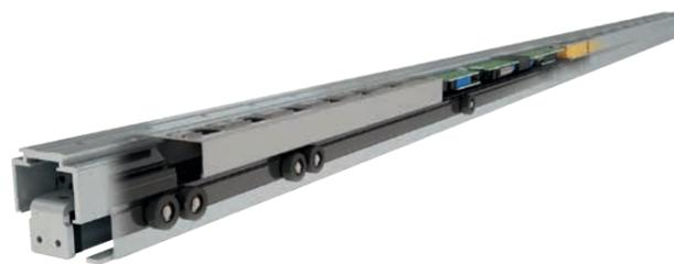
E-MOTION is the linear motorised unit for ECLISSE sliding pocket doors: the door opens and closes by itself. The magnetic technology applied makes it very silent and easy to install. The motor unit is pre-assembled with power supply and switch cables, ready to be installed.
