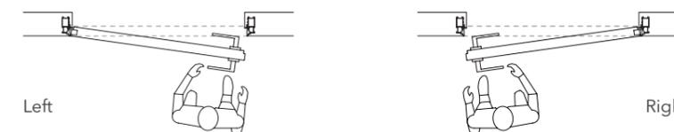
ECLISSE SYNTESIS® LINE BATTENTE INCLINED can be realized with different angles ( $\alpha$ ), both with or without header.
