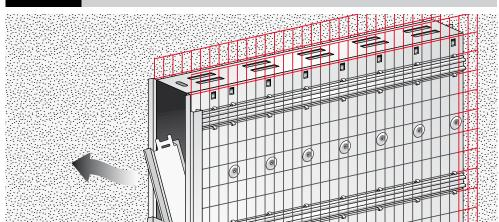
Insert the metal tongues at the end of the top beam into the slots at the top of the metal door post.
